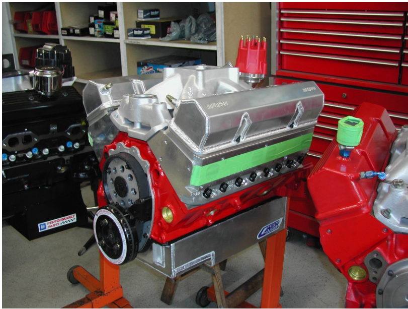
380 Cubic Inch Small Block Chevy 704HP at 8400RPM
